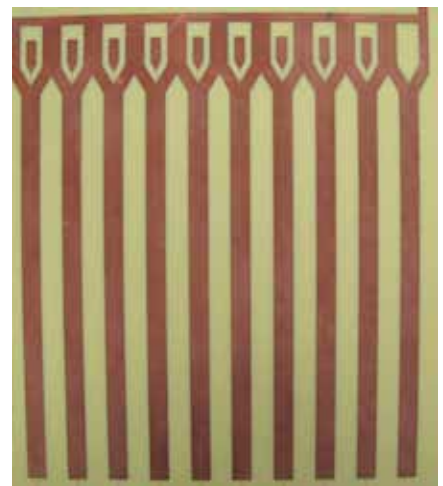
Figure 1. Bono test board.
