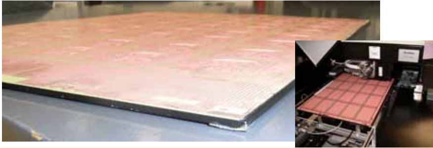
Figure 8. Substrate flattened by support carrier.
