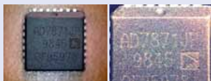
A. The original part, and the part after solvent testing.
