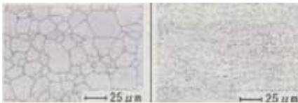
Figure 4. Grain size comparison: SS 300 series (left) and new material (right).
