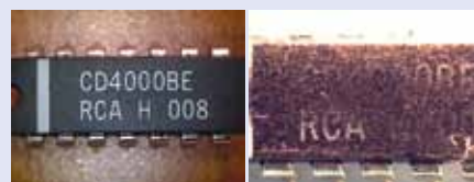
A. The original part, and blacktop removed by solvent testing.
