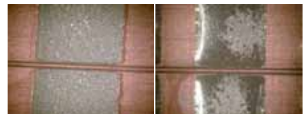
Figure 2. Solder paste after printing (left) and after reflow (right).
